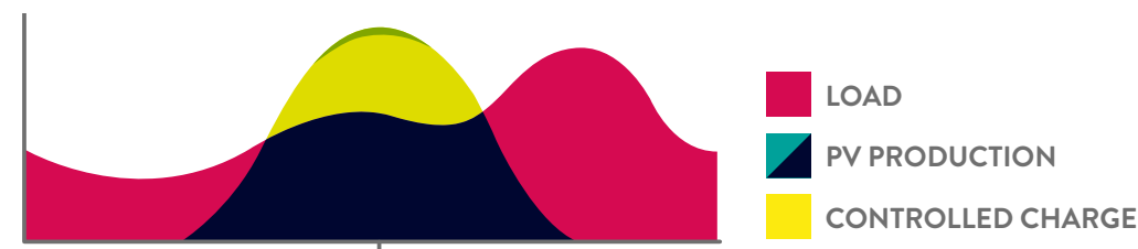
Charge control: Electric vehicle only charges when a surplus of solar power is available.
